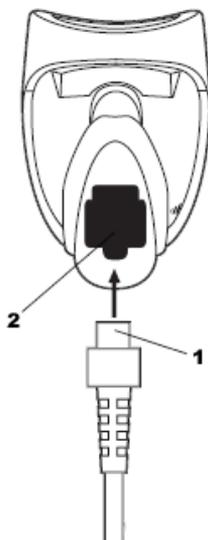
2. Gently tug the cable to ensure the connector is properly secured.
